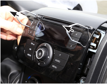
2. Insert special radio release keys into holes of OEM head unit and pull out OEM head unit (see arrows)
