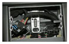
2. Remove middle bar to clear space for double DIN navigation
