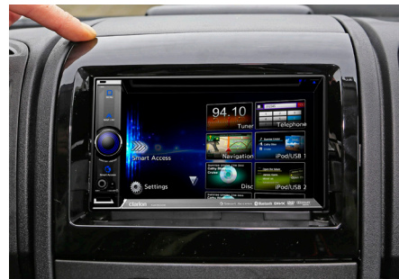
8. Put fascia plate over double DIN head unit to finish installation
