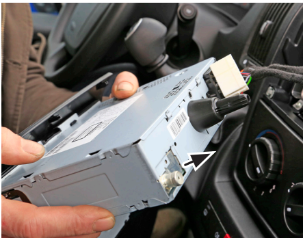
3. Unplug all cables and remove OEM head unit
